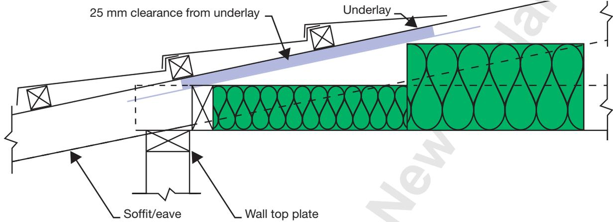
Figure 22 – Roof detail for a low-pitch roof
