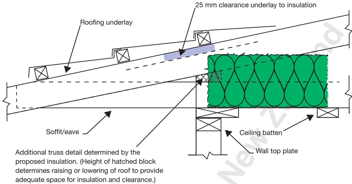
Figure 24 – Low-pitch roof with metal tiles
