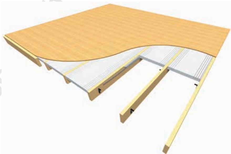
Figure 31 – Installation of underfloor rigid sheet floor insulation
