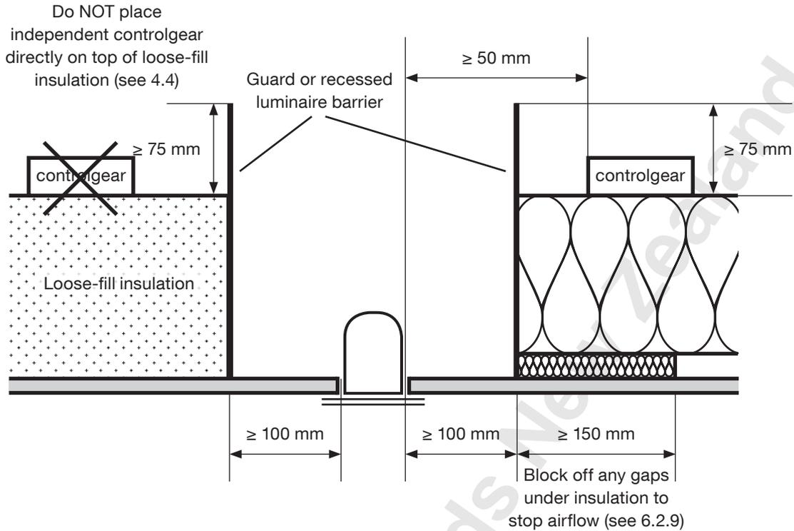
**Figure 8 – Installing ceiling insulation around recessed luminaires that are NOT of the type CA 80, CA 90, CA 135, IC, IC-F, or IC-4 where insulation is NOT secured in position or where insulation is loose-fill and where the luminaire manufacturer’s instructions are not known**
