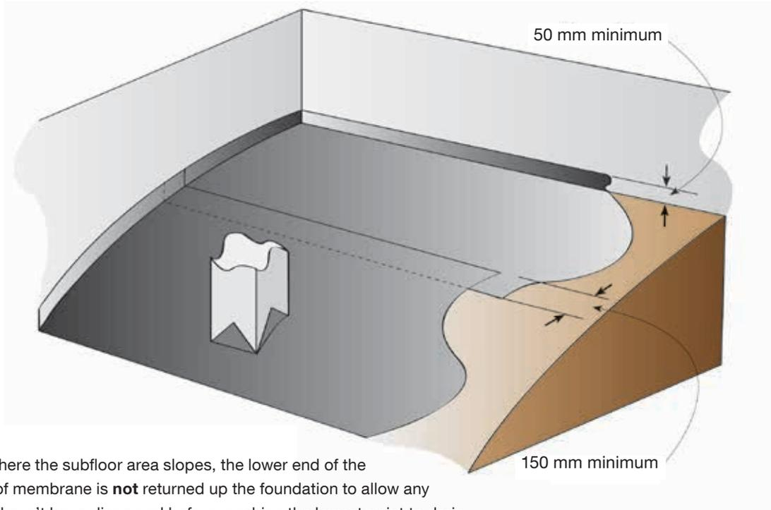
NOTE – Where the subfloor area slopes, the lower end of the damp proof membrane is **not** returned up the foundation to allow any water that hasn't been dispersed before reaching the lowest point to drain.
