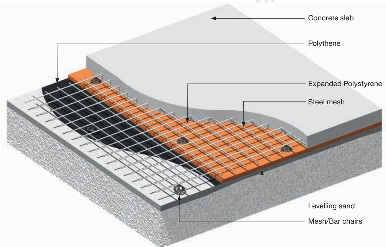
Figure 36 – Under-slab insulation
