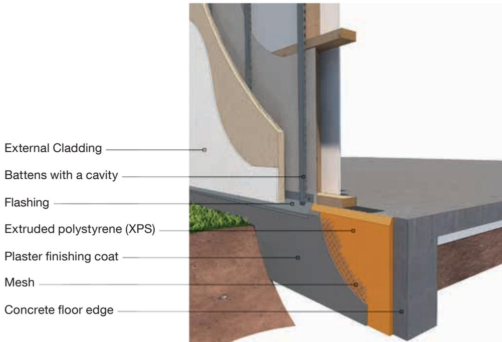
Figure 37 – Slab perimeter insulation
