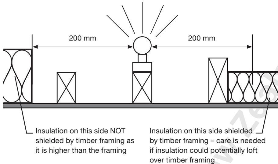
On the left hand side the top of the ceiling joist is lower than the top of the insulation and does not fully shield the insulation. The full clearance needs to be maintained. On the right hand side a smaller clearance is acceptable as the insulation is fully and permanently shielded by timber framing (provided the insulation material cannot potentially loft over the top of the ceiling joist – where this is not guaranteed the full 200 mm clearance shall be maintained).
